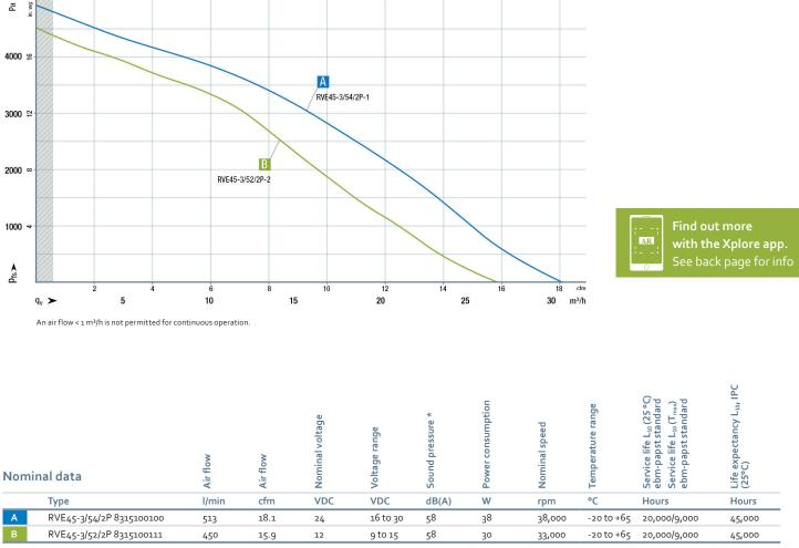
\* Extraction noise @ 1,000 Pa. Blower with open intake side facing upwards, opposite side lays on 10 cm thick foam, outlet openings with hose and 4 mm standard nozzle (acoustically insulated),
